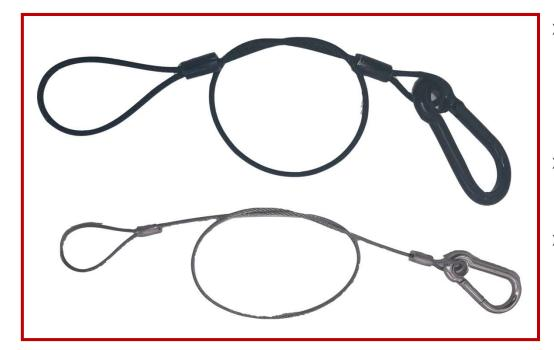
These Safety cable with Carabiner has a 5/16" carabiner clip on one end and a loop on the other. Safety cable provides an extra layer of safety and prevents objects from falling in the event that a clamp should fail or is improperly tightened. Safety Cable with Carabiner prevent hazard, especially when lights are hung overhead on a pipe or grid.
